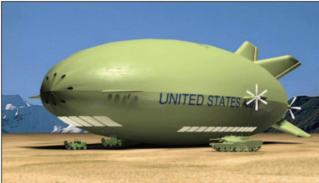
Figure 2 Early Suggested Design for the WALRUS HTA Airship
